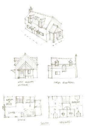
An example of the sketches provided as part of an 'Initial Design & Feasibility Study' into a new house, showing sketch floor plans, 3D view and principle elevation.
